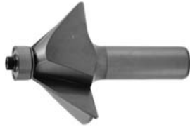
RB1520655 45 Degree Chamfer Bit 1" Cutting Height 1/2" Shank 2 Flutes 1 Bearing
