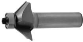
RB1520625 45 Degree Chamfer Bit 5/8" Cutting Height 1/2" Shank 2 Flutes 1 Bearing
