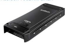
5ch hybrid design 2) AB Class output  $(2 \times 250 \text{w RMS } 4\Omega)$  2) A Class outputs  $(2 \times 75 \text{w RMS } 4\Omega)$  1) D Class output  $(1 \times 1000 \text{w RMS } 2\Omega)$  LED status display
