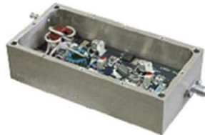
PM1-525-10 1 - 525 MHz amplifier module Pout=10w
